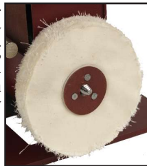
Buffing mop & pigtail mandrel Screwed onto the pigtail mandrel, the loose leaf cotton mop will produce a highly polished finish on any tool when used in conjunction with the honing paste
