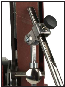
Fingernail profile arm* Maintain the desired fingernail profile on any spindle & bowl gouge from 1/4" (6mm) - 3/4" (19mm)
