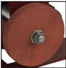
Honing wheel & arbor Fixed to the accessory attachment hub using the arbor the rubberised honing wheel that can be shaped to suit any tool
